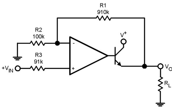
$V_O = 0$   $V_{DC}$  for  $V_{IN} = 0$   $V_{DC}$ ,  $A_v = 10$
