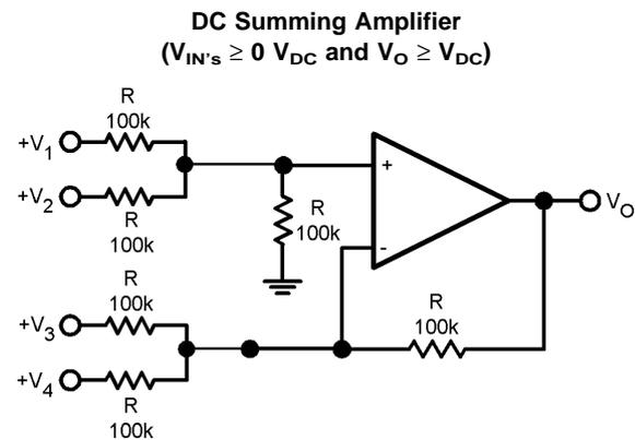
Where:  $V_O = V_1 + V_2 - V_3 - V_4$ , ( $V_1 + V_2 \geq V_3 + V_4$ ) to keep  $V_O > 0$   $V_{DC}$
